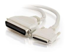
This Ultra2/Ultra3 LVD/SE external VHDCI (Very high density Cable Interconnect) cable features 28 AWG double-shielded twisted-pair cabling, ferrites and 0.8mm 68-pin molded connectors to reduce EMI/RFI interference. Designed to meet or exceed SCSI specifications, this cable is primarily used to connect advanced SCSI multiport applications to RAID controllers, and is built with the offset connector so that it may be used in stacking environments.
