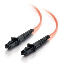
With MTRJ to MTRJ termination, this high quality fiber optic patch cable is specifically designed for ethernet, multimedia, or communication applications. The MTRJ connector features an easy-to-use latch-type design similar to the RJ connector on a Cat5 patch cable, and is half the size of the SC connector. With its small footprint design, the MTRJ connector can increase the port density.
