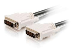
This precision-engineered cable is fully compliant with the DVI standard defined by DDWG (Digital Display Working Group). The DVI-D dual link configuration provides enough bandwidth for resolutions up to 2560x1600 pixels and allows high speed digital video transmission up to 9.9 Gbps. 28 AWG copper conductors are individually insulated in foam-polypropylene to minimize crosstalk, and ensure high speed, error-free transmission.
