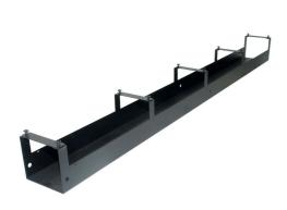
This cable raceway is constructed from 0.062in aluminum, and is designed to install between an APW modular networking frame and a cable management rack. Featuring swing-away and removable cable retainers, this raceway has grommeted edges for cable protection. All joining hardware is included.
