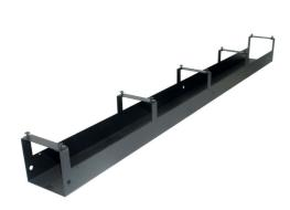
This cable raceway is constructed from 0.062in aluminum, and is designed to install between an APW modular networking frame and a cable management rack. Featuring swing-away and removable cable retainers, this raceway has grommeted edges for cable protection. All joining hardware is included.
