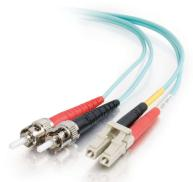
This USA made OM3 Duplex Multimode Fiber Optic Cable is ideal for connecting 10GBase-SR, 10GBase-LRM, SFP+ and QSFP+ tranceivers for 10 gigabit network connections. This cable has a OFNR-rated jacket allowing it to be used in a riser application. This cable also provides backward compatibility with existing 50/125 equipment and the performance headroom required to support LED and VCSEL laser light sources, and 10 gigabit ethernet applications.
