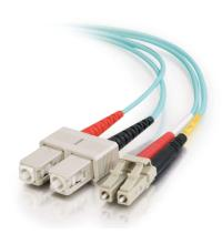
This USA made OM3 Duplex Multimode Fiber Optic Cable is ideal for connecting 10GBase-SR, 10GBase-LRM, SFP+ and QSFP+ tranceivers for 10 gigabit network connections. This cable has a OFNR-rated jacket allowing it to be used in a riser application. This cable also provides backward compatibility with existing 50/125 equipment and the performance headroom required to support LED and VCSEL laser light sources, and 10 gigabit ethernet applications.
