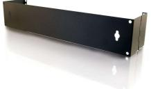
When minimum space is required, this heavy duty 16 AWG steel bracket is a great alternative to a full-sized rack. Designed for standard 19-inch patch panels, the bracket's hinged design enables convenient wallmounting of patch panels and small equipment while it saves valuable floor space. The bracket provides universal mounting for right or left hinging. Has a black powder coat finish. For EIA spacing, it accepts either 10-32 or 12-24 screws.
