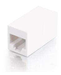
This coupler provides a female-to-female feed-through connection to extend the length of two Cat5E patch cables. Capable of handling LAN speeds up to 100 Mbps, this coupler meets TIA/EIA 568A specifications and is Power Sum Certified. Use for straight-through RJ45 Cat5E data applications.
