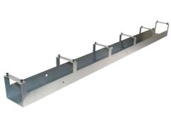
This cable raceway is constructed from 0.062in aluminum, and is designed to install between an APW modular networking frame and a cable management rack. Featuring swing-away and removable cable retainers, this raceway has grommeted edges for cable protection. All joining hardware is included.
