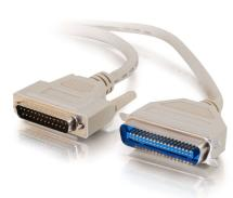
Engineered with high quality connectors and a specialized wire type, these parallel printer cables provide an increased data rate and two-way communication of IEEE-1284-compliant printers and scanners. These parallel printer cables enable high speed, bi-directional communication between a desktop PC and a peripheral. Foil shielding and coverage braid provide maximum resistance against harmful EMI/RFI, and help to achieve the maximum performance from attached peripherals.
