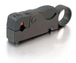
Primarily for f-type connectors that require the cable to be stripped to two different lengths. This tool strips in four lengths: 4, 6, 8, and 12mm. Use it for RG174, RG58, RG59, and RG6 (dual or quad shield) cable. Its spring-loaded jaws hold the cable while a rotating motion precisely strips the outer jackets.
