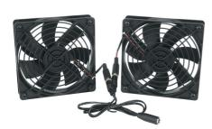
Fan kits for the Vertical wall mount include (2) 115VAC fans, power and grounding cord, fan guards, and hardware needed for installation. Fans deliver 85 CFM each and provide active cooling for wall mount cabinets.
