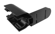
Designed to be integrated with the Legrand Q-Series vertical manager, the bend limiting/cable management clip allows both fiber and copper to be dressed in the same vertical manager while safely separating them. The bend limiting clip portion ensures proper radius for fiber and the front fence section easily attaches copper bundles.
