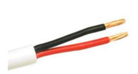
This is the right cable to install audio throughout your house. Made from 41 strands of 99.9% high-purity copper, this speaker wire is very flexible and less likely to kink during installation. CL2-rated for use inside walls, this wire features a flame-retardant white PVC jacket that helps to diminish the potential of fire spreading between floors.
