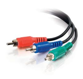
Component video cables bypass a TV's Y/C separator and color decoder, routing the color (Y/Pr/Pb) information directly into the TV's matrix decoder. By sending the pure DVD component video signal directly to a component video input-equipped display device, the DVD signal forgoes the extra processing that normally would degrade the image. The result is a vastly increased image quality, with incredibly lifelike colors and crisp detail.
