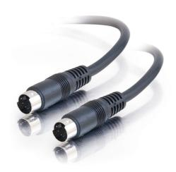
Our s-video cable is constructed from high quality multiple conductors that deliver high quality video images. Separate conductors carry the Y-component (Chrominance) separately from the C-component (Luminance), to provide higher resolution and better picture quality than a composite video cable. Molded connectors with integrated strain relief; flexible PVC jacket.
