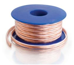
This cost-effective wire provides maximum sound for your dollar. Clear PVC jacket with white marker enables easy polarity identification. The high strand count offers maximum flexibility for easier installations. For the two 18 AWG conductors, each conductor is manufactured from 3 bundles of 24 copper strands. Cross section of the wire is 0.10in x 0.20in.
