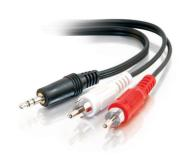
Our audio y-adapter cable splits an audio signal or adapts from one connection to another to meet your application needs. This cost-effective cable is quality-made to deliver crisp, clear sound for less. Brass/nickel-plated plugs connect to 26 AWG spiral-wrapped copper-shielded wire. The dual conductor is shielded to protect against EMI/RFI interference. The connectors are fully molded to provide excellent strain relief for durable use.
