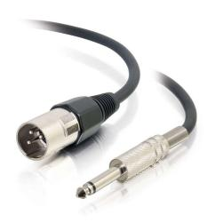
Use this XLR to 1/4in cable to connect unbalanced sources to balanced XLR inputs. This pro-audio cable is made from 22 AWG twisted pair audio cable under an aluminum foil shield and 60% copper braid for maximum shielding from noise. The highly flexible 7mm PVC jacket reduces the risk of the cable kinking and damaging the conductors.
