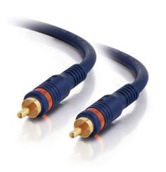
The Velocity digital audio cable is a great upgrade to the cables typically included with consumer electronics products. The low-loss 75 0hm oxygen-free copper center conductors and foam dielectric provide high quality digital sound and performance. The 100% aluminum foil and dual OFC braid shields protect against unwanted noise and interference.
