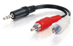
Our audio y-adapter cable splits an audio signal or adapts from one connection to another to meet your application needs. This cost-effective cable is quality-made to deliver crisp, clear sound for less. Brass/nickel-plated plugs connect to 26 AWG spiral-wrapped copper-shielded wire. The dual conductor is shielded to protect against EMI/RFI interference. The connectors are fully molded to provide excellent strain relief for durable use.
