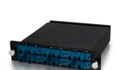
Small form factor:  $1.125in \times 5.125in \times 4.5in$ . This breakout module provides the mechanical distribution of the 12-strand MTP/MPO connector. Housed in a rugged steel enclosure guaranteed for life, this durable module arrives fully loaded with the preterminated and tested MTP/MPO breakout harness. It is shipped with a test report that can assist in calculating the optical budget.
