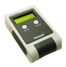
The high-tech LANsmart TDR Cable Tester detects, locates, and displays basic wire connection problems including opens, shorts, miswirings, reversals, split pairs and shield continuity for RJ45, Cat5, Cat6, UTP and STP. Plus, it measures cable length for UTP and STP cable without remotes by using TDR (Time Domain Reflectometer) technology in real time. LANsmart displays the results in a pin-to-pin format.
