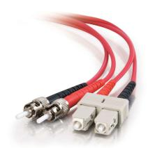
With SC to ST termination, this high quality fiber optic patch cable is specifically designed for ethernet, multimedia, or communication applications. The SC connector features a push-pull locking system while the ST connector features a bayonet locking system.
