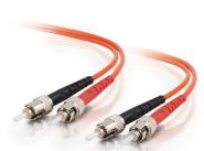
With ST to ST termination, this high quality fiber optic patch cable is specifically designed for fast ethernet, fiber channel, ATM  $and\ gigabit\ ethernet\ applications.\ The\ ST\ connector\ features\ a\ bayonet\ locking\ system.\ The\ LSZH\ jacket\ is\ composed\ from$ materials that lessen the smoke and halogen emissions when the cable is exposed to extreme temperatures.
