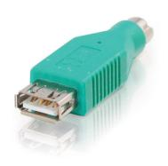
This adapter connects your USB keyboard or mouse to a PS/2 port on your computer. Simply plug this compact adapter into any PS/2 port, then connect your mouse or keyboard.
