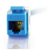
Designed for superior performance, this keystone jack is available in several colors to match housing or allow color-coded port designation in compliance with TIA-606 requirements. Includes 110-type IDC termination with strain relief caps, and comes standard with 50 µinch gold plating on the jack contacts.
