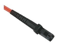
With MTRJ to SC termination, this high quality fiber optic patch cable is specifically designed for ethernet, multimedia, or communication applications. The MTRJ connector features an easy-to-use latch-type design similar to the RJ connector on a Cat5 patch cable, and is half the size of the SC connector. With its small footprint design, the MTRJ connector can increase the port density. The SC connector features a push-pull locking system.
