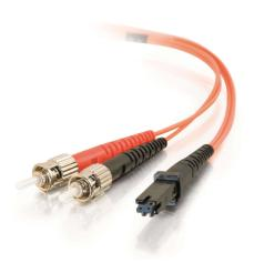
With MTRJ to ST termination, this high quality fiber optic patch cable is specifically designed for ethernet, multimedia, or communication applications. The MTRJ connector features an easy-to-use latch-type design similar to the RJ connector on a Cat5 patch cable, and is half the size of the SC connector. With its small footprint design, the MTRJ connector can increase the port density.
