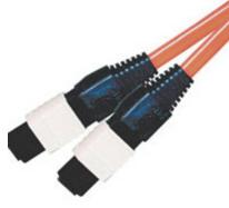
Make MTP/MPO your choice for high density fiber networks; it's specifically designed for fast ethernet, fiber channel, ATM and gigabit ethernet applications. Save time and money with MTP/MPO's increased ease of installation - simply pull one cable rather than twelve. Each MTP/MPO fiber assembly consists of twelve laser-optimized, 62.5/125 multimode fibers under one OFNP plenum-rated jacket.
