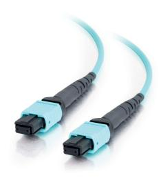
Make MTP/MPO your choice for high density fiber networks; it's specifically designed for fast ethernet, fiber channel, ATM and gigabit ethernet applications. Save time and money with MTP/MPO's increased ease of installation - simply pull one cable rather than twelve. Each MTP/MPO fiber assembly consists of twelve laser-optimized, 10G 50/125 multimode fibers under one PVC (OFNR-rated) jacket.
