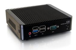
The Network Controller for HDMI over IP is a Linux-based PC that allows users to control HDMI over IP products, supporting video wall and multiview connectivity. The Network Controller may be managed via a Web interface or the C2G AVoIP Control Smartphone & Tablet App.
