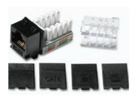
Designed for superior performance, this keystone jack is available in 9 colors to match housing or allow color-coded port designation in compliance with TIA-606 requirements. Includes 110-type IDC termination with strain relief caps, and comes standard with 50 inch gold plating on the jack contacts.
