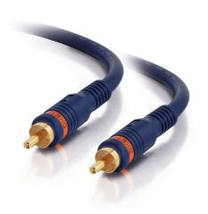
The Velocity digital audio cable is a great upgrade to the cables typically included with consumer electronics products. The low-loss 75 Ohm oxygen-free copper center conductors and foam dielectric provide high quality digital sound and performance. The 100% aluminum foil and dual OFC braid shields protect against unwanted noise and interference.
