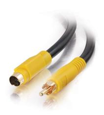
Connect s-video devices (your laptop, PC or game console) to a TV without an s-video port. This bi-directional video cable converts a composite RCA signal to s-video or vice versa without using couplers that can cause signal loss. Quality 75 Ohm coax cable is double-shielded with 85% alumimum foil and braid to reduce unwanted noise and distortion.
