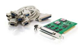
This PCI bus 8-port serial board, with a fan-out (octopus) cable, configures 8 COM ports on the faster PCI bus, at data rates up to 115.2 kbps. It is an extremely dependable communication solution for ISPs or any type of RAS system that does not deal with an overwhelming amount of traffic. Each port includes integrated 16-byte FIFO buffer with software-configurable Tx/Rx triggers.
