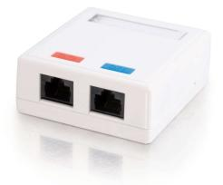
Ideal for surface mount applications, especially in confined spaces. Mount for either side or base entry of cables. Boxes come with mounting screws and adhesive tape, and a cable tie for strain relief. The snap-on cover enables easy closure or access for quick installation. Each box includes a write-on label with holder for easy designation of different system or station. Contacts are phosphor bronze plated with 50 inch hard gold.
