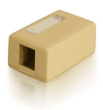
Ideal for surface mount applications, especially in confined spaces. Mount for either side or base entry of cables. Boxes come with mounting screws and adhesive tape, and a cable tie for strain relief. The snap-on cover enables easy closure or access for quick installation. Each box includes a write-on label with holder for easy designation of different system or station.
