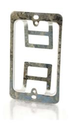
Mounting a flush-mount wall plate without a back box is easy. This bracket inserts into the wall opening, with the flexible tabs bending upward to secure the bracket to the opening. Standard screw holes accept all wall plate configurations. Compatible with NEMA standards, this bracket works with all standard size single gang wall plates.
