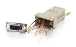
Using modular adapters with inexpensive silver satin or flat oval twisted pair wire has become a standard way to run client server applications. Needing to connect dumb terminals on the desktop back to a central patch panel or directly to a MUX via RS-232, many network planners have implemented modular adapters as the most cost-effective way to complete the connections.
