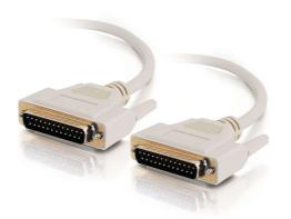
All 25 lines are wired straight through pin-to-pin for ease of compatibility. Each cable is foil shielded for EMI/RFI protection, and is available fully molded with thumbscrew connectors for a fast, easy connection every time.
