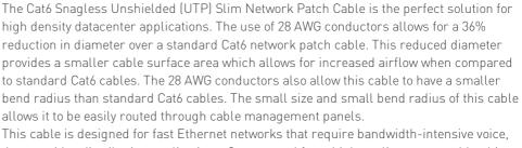
This cable is designed for fast Ethernet networks that require bandwidth-intensive voice, data, or video distribution applications. Constructed from high quality copper cable, this design minimizes Near-End Crosstalk (NEXT) levels. The molded, snagless boot prevents unwanted cable snags during installation and provides extra strain relief. Available in a variety of colors to easily color-code your network installation.
