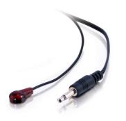
Ideal for use with #40430, Remote Control Repeater Kit. Plug this IR emitter into a 2-conductor 3.5mm keystone jack and stick it over the IR eye on your audio/video equipment. The emitter operates on 12 VDC and is compatible with most IR devices. Put your components where they belong, not where you see them! You can even control audio/video devices located behind doors or in other rooms.
