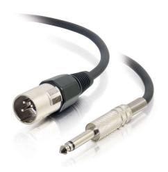
Use this XLR to 1/4in cable to connect unbalanced sources to balanced XLR inputs. This pro-audio cable is made from 22 AWG twisted pair audio cable under an aluminum foil shield and 60% copper braid for maximum shielding from noise. The highly flexible 7mm PVC jacket reduces the risk of the cable kinking and damaging the conductors.
