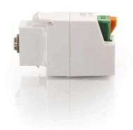
This 3.5mm keystone module snaps into standard keystone wall plates to allow you to connect IR targets into the IR control system. Connect a 3.5mm stereo cable from your PC sound card and play stereo sound throughout your distributed audio system. 3.5mm modules are easy to connect to UTP cable; simply push the terminal and insert the wire.
