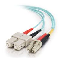
This OM3 Duplex Multimode Fiber Optic Cable is ideal for connecting 10GBase-SR, 10GBase-LRM, SFP+ and QSFP+ tranceivers for 10 gigabit network connections. This cable has a 0FNP-rated jacket allowing it to be used in a plenum application. This cable also provides backward compatibility with existing 50/125 equipment and the performance headroom required to support LED and VCSEL laser light sources, and 10 gigabit ethernet applications.
