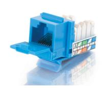
Designed for superior performance, this keystone jack will work with C2G, formerly Cables To Go, wall plates and surface boxes or any standard keystone and angled multimedia wall plate or patch panel. Available in 9 colors to match housing or allow color-coded port designation in compliance with TIA-606 requirements. Each keystone jack includes 110-type IDC straight-back termination with strain relief caps, and comes standard with 50 [micro]inch gold plating on the jack contacts.
