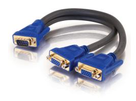
The Ultima SXGA cable optimizes style, quality, and value in a cable specially designed for high performance. This y-cable splits the VGA signal to provide simultaneous display of the same picture. It is constructed from 3 individually-shielded 75 0hm coax and 4 twisted pair cable to minimize crosstalk, noise, and other EMI/RFI interference.
