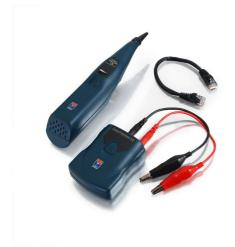
This kit consists of the CT10 toner/blinker, the CT15 tone probe, the CC2 carrying case, and one RJ45 jumper cord; it is specifically designed for network managers and technicians. Toning an active LAN circuit can disrupt network traffic and is difficult to track due to cable twist and tone bleed. This test system works with both active and inactive (dark) cables, and features a port ID function that blinks the link light to verify cable connectivity.
