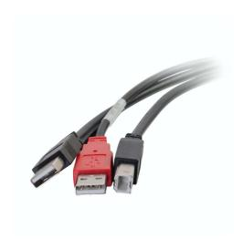
When a standard USB cable cannot transfer enough power to operate an external device, such as a portable 2.5in hard drive, you need a USB 2.0 y-cable. Simply plug this cable's USB B end into the device, and then plug the two USB A ends into open USB ports on one PC or Mac. This cable then pulls power from both USB ports, and thus increases the output to the external drive.
